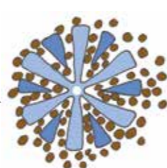
CROSS-SECTION OF MICROFIBRE
